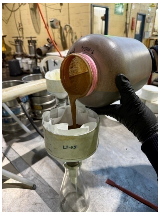
Figure 9.3: Oxide Master Composite from Cyanidation Leach Test being filtered showing low to moderate viscosity
