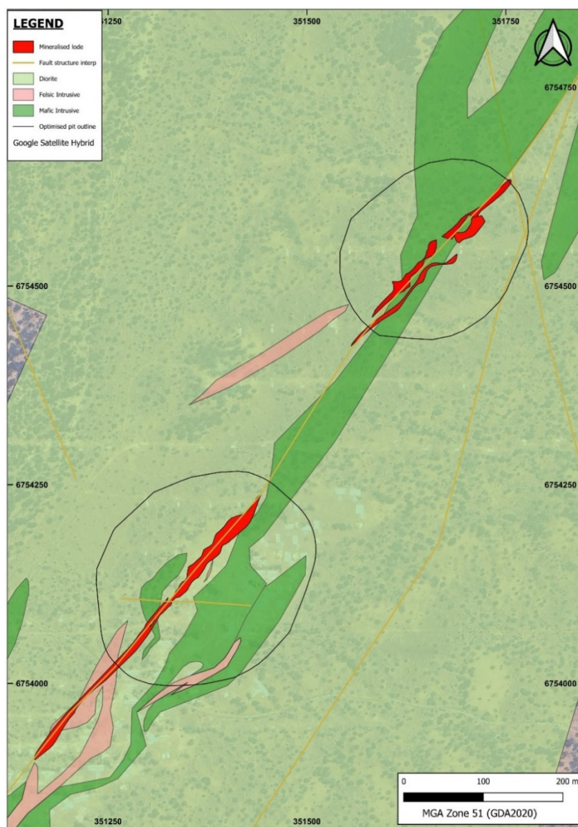
Figure 3.5: 2D geological interpretation of Swiftsure and Tiptoe deposits
