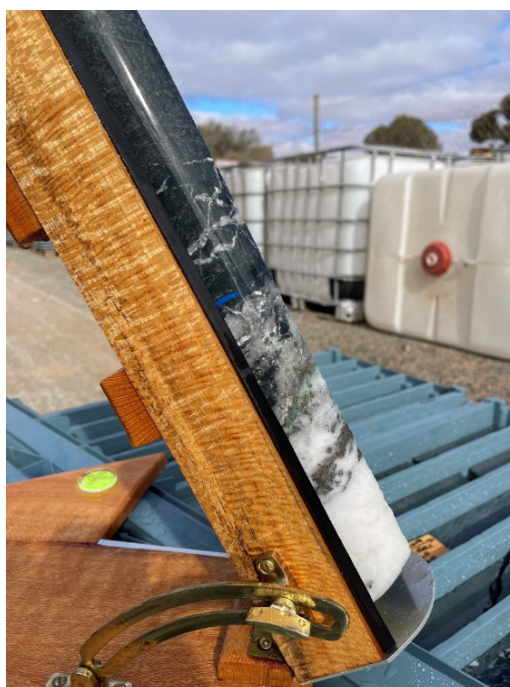
Figure 3.6: Showing drillhole MERC021 @ ~338m spatially orientated, looking SW showing the mineralised veining in hanging wall to dolerite/diorite contact, returning grades 0.5m @ 48.8g/t.
