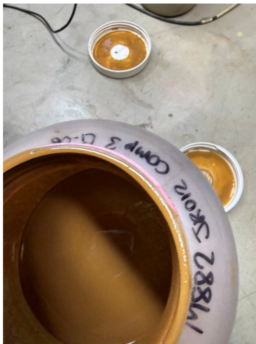
Figure 9.2: Oxide Master Composite Sample from Cyanidation Leach Test showing low to moderate viscosity
