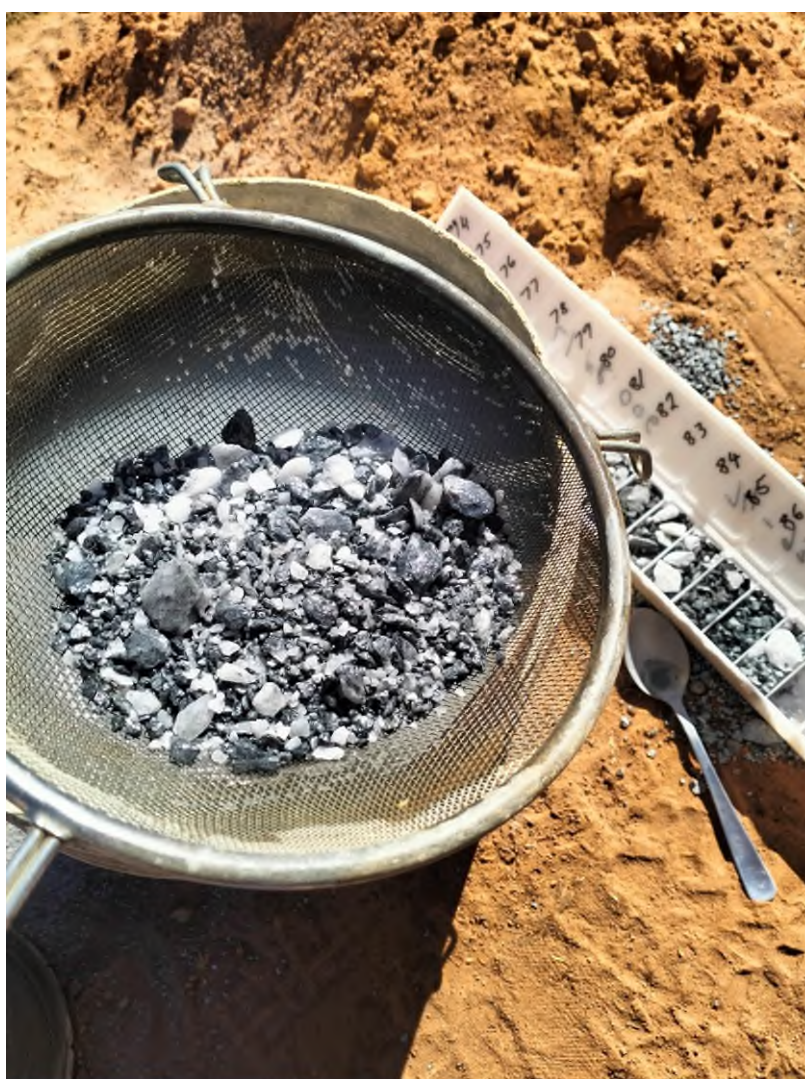
Figure 3. Swiftsure high-grade zone with typical grey quartz, minor sulphides and gold - 2m @ 17.4g/t from 88m in RC L1.FR.006
