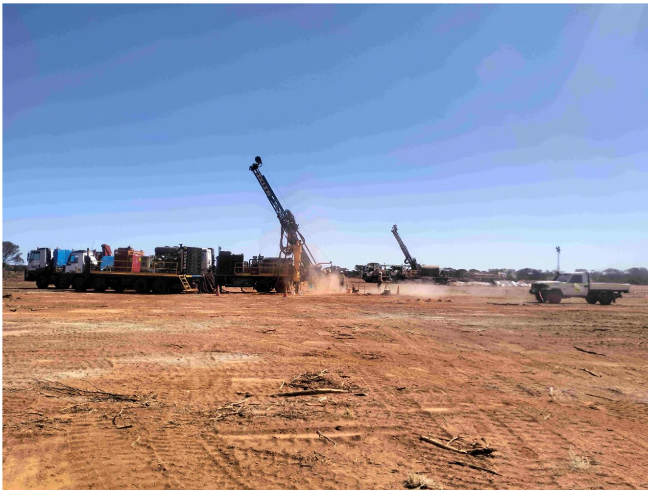
Figure 2, RC and Diamond Drilling onsite at the Swiftsure proposed pit site.
