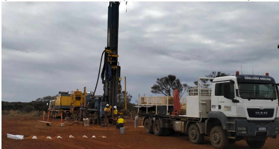
Figure 1, Challenge drilling onsite at Swiftsure with RC rig
