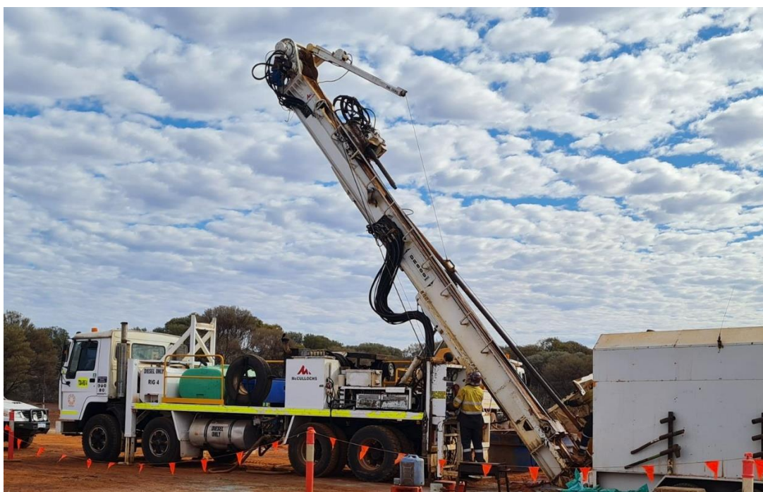
Figure 1: Topdrive diamond drilling at Kookynie Gold Project
