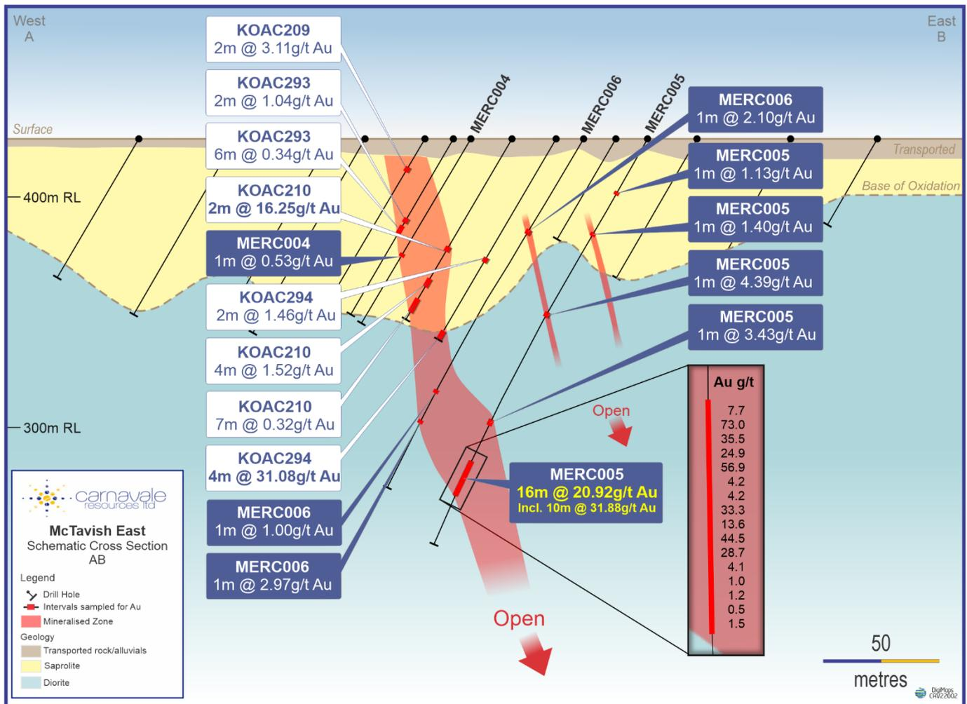
**Figure 4: Cross section 6753880mN through mineralised zone at McTavish East**
